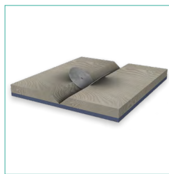
Milling one groove into only the substrate
