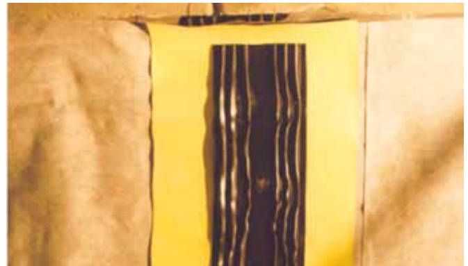
Geomembranes with welded water stops produced in prefabrication
