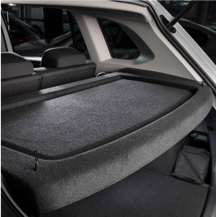
Hutablage aus RENOLIT TECNOGOR . (Foto: RENOLIT COMPOSITES , PR002)
