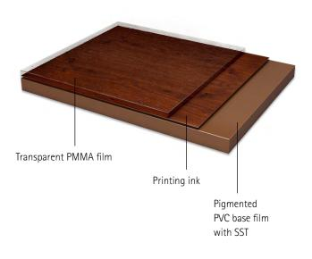
Diagram showing the structure of the exterior film RENOLIT EXOFOL MX
