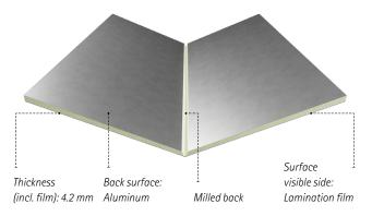
Processing the high-quality cladding panel is extremely simple: mill a small groove into the back of the panel and you can bend RENOLIT BENDIT to the exact angle you need. Any angle up to 90 degrees is possible. The fold is positioned exactly where you want it, and the beautiful surface can withstand it all.
